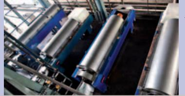
◆ D3 PRO in action Since 2009 a D3 PRO process incorporating 3-phase decanters has been clarifying and purifying crude palm oil at a Malaysian oil mill with a total capacity of 80 tons FFB/h.
