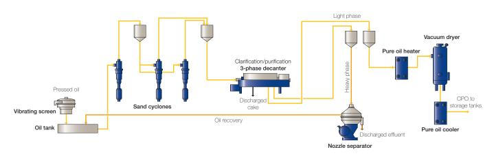
D3 PRO process with 3-phase clarification/purification and oil recovery
