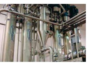
The lecithin is then separated from the vapours in a large cyclone, under vacuum, before being sent to Contherm heat exchanger(s) for cooling with water.
