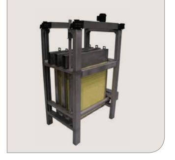
The Alfa Laval AS-H Iso-Disc Cloth Media Filter is engineered as a continuous operating process that utilizes a fixed cloth media and an efficient linear backwashing system that cleans the media equally across the whole surface area. The cloth media is fully submerged into a tank to allow 100% use of filtration area at all times.
